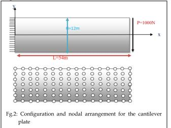
First, we studied the effect of the parameters of the radial basis functions RBF-MQ and the sizes of support and quadrature domain on convergence of the LRPIM method:
