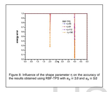
We have also used the radial basis function RBF-TPS to study the convergence of LRPIM method:
